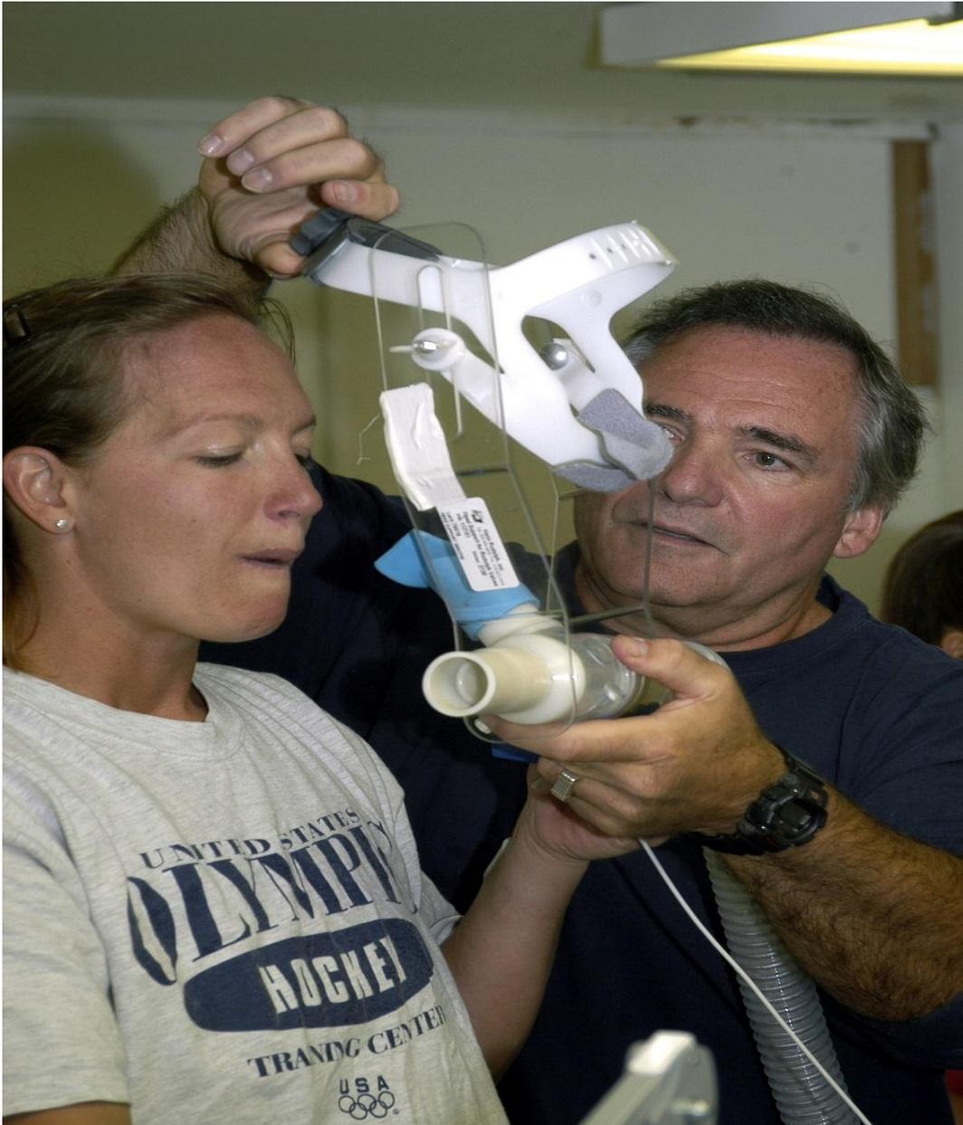
Figure-1. The original hans rudolph valve and mouthpiece.
