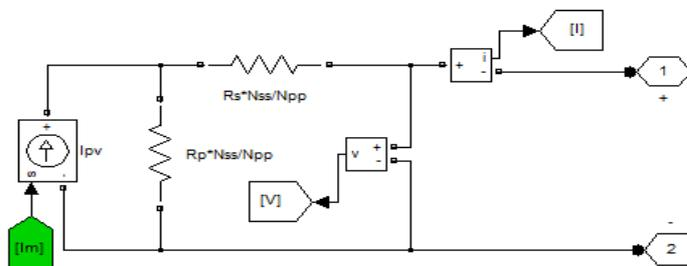
In order to create the input supply or model current  $I_m$ , to the equivalent circuit of PV, firstly the saturation current of  $I_o$  was developed. This is done by using the following equation of 1, 2 and also with the selected parameters. Then the mathematical model of  $I_o$  was developed in Matlab/Simulink as shown in Figure 4.
