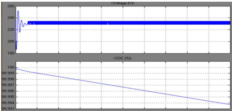
Figure 12 shows output voltage buck converter in DC volts. Here the voltage from PV 240V are fluctuated and buck converter are used to get pure DC voltage.
