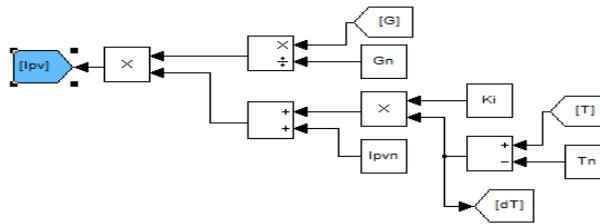
Finally both parameters of  $I_o$  and  $I_{pv}$ , also with the selected parameter were inserted in equation of 4 in order to obtain the input supply of  $I_m$ . Then the mathematical model of  $I_{pv}$  was developed in Matlab/Simulink as shown in Figure 6.
