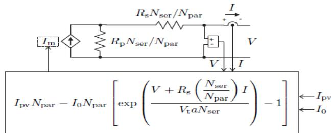
**Figure-3.** Equivalent model of PV system in Matlab Simulink with input  $I_m$  and output port that connect to outside of subsystem.
