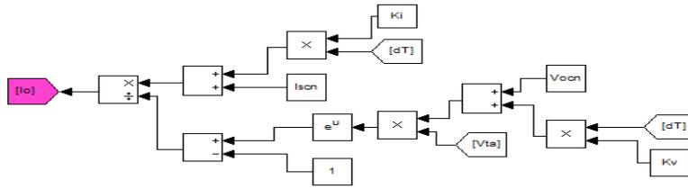
Then the light generated current  $I_{pv}$  was developed by using equation 3 with the selected parameters. Then the mathematical model of  $I_{pv}$  was developed in Matlab simulink as shown in Figure 5.
