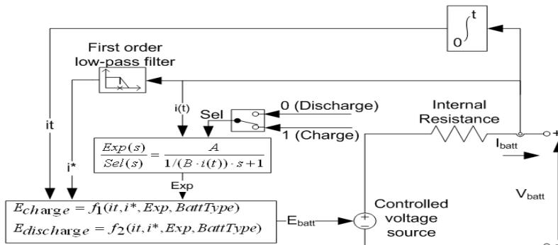
Lead acid model for discharge model with selected parameter was inserted in equation 9. While for charge model with selected parameter was inserted in equation 10.
