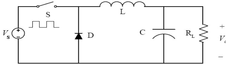
Duty ratio  $D$ , with desired output voltage  $V_o$  and voltage input  $V_s$
