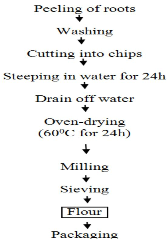
Fig-1. Flow chart for processing sweet potato roots into flour.
