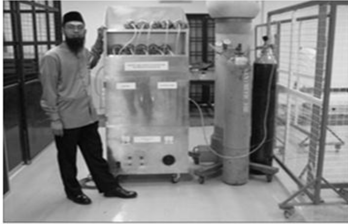
Fig-2. Ozone treatment system
