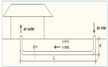
Figure-1. Schematic diagram of the earth-air-pipe heat exchanger.
