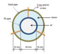
Figure-4. A cross-section of the insulated hybrid materials.
