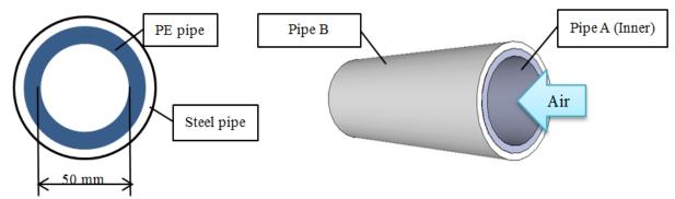
**Figure-3.** A cross section of two pipes in a hybrid pipe system
