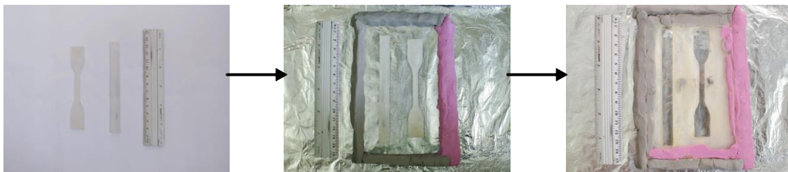
Fig-2. Sequence of preparing the mould for the samples for mechanical testing
