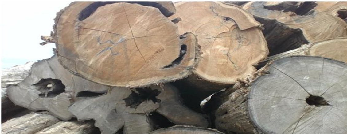
Plate-1. Rotted heart of teak harvested by the customer from Mtibwa plantation
