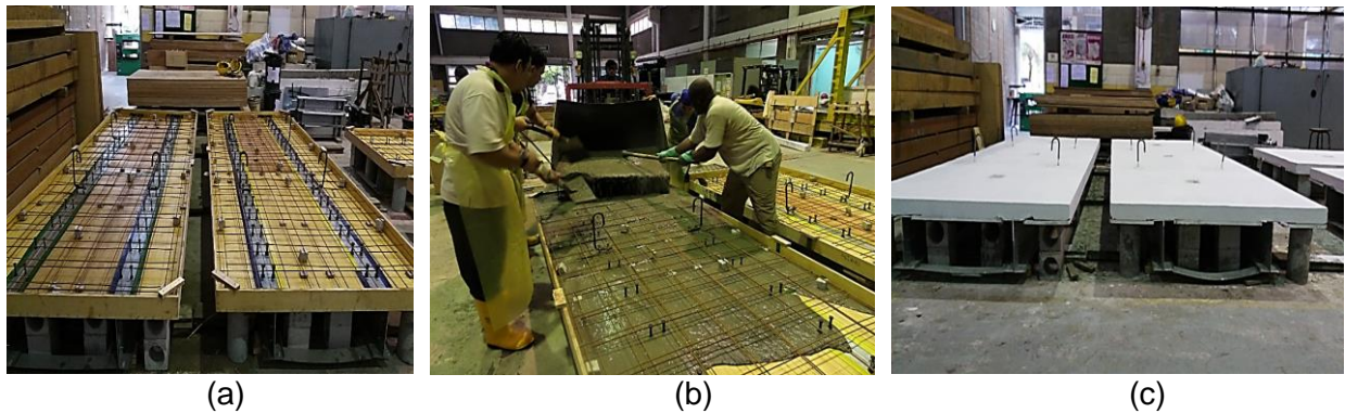
Figure-2. Preparation of full-scale test specimens [(a) samples formwork, (b) samples casting, (c) finished samples]
