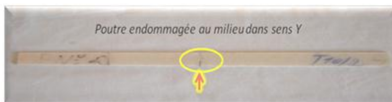
Fig-2. Pre- defect beam in the middle
