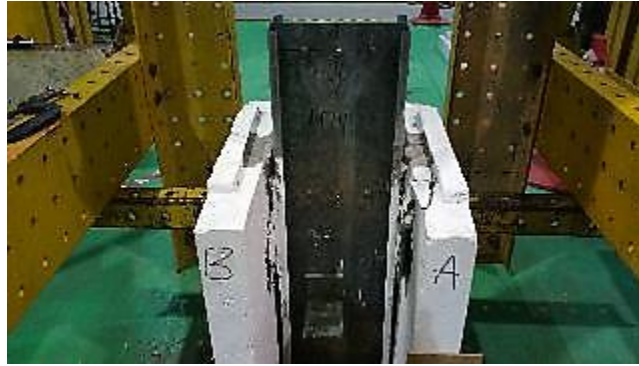
Figure-7. Failure mode of S4M14 test specimen
